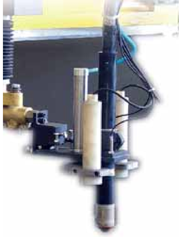
collision-sensor-and-initial positioning device
