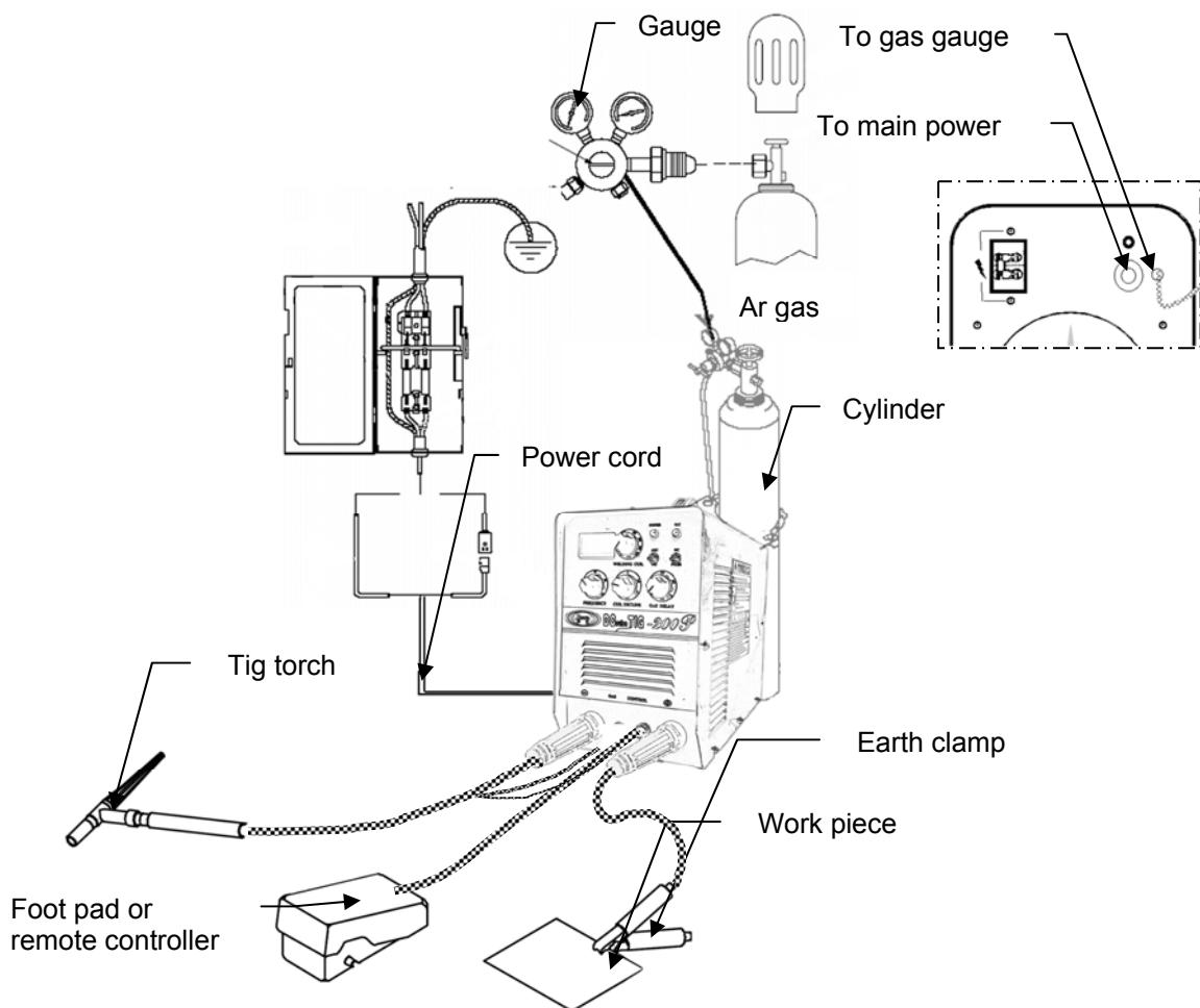
Figure 2.1      Tig welding connection diagram
