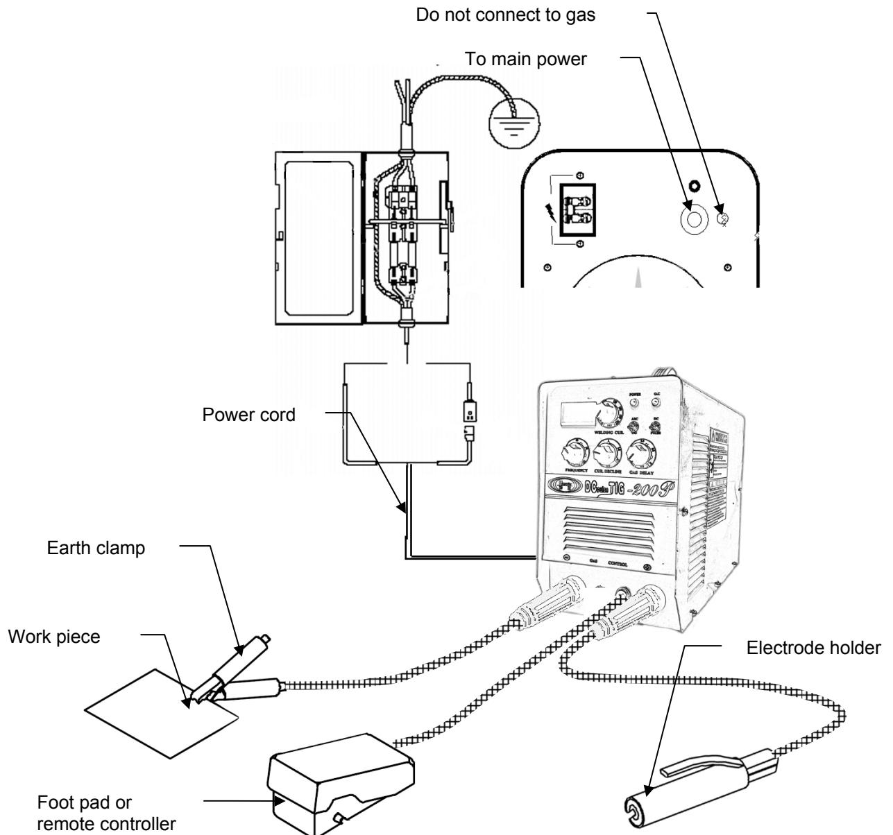
Figure 2.2 Arc welding connection diagram
